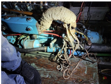
A crude example of a swan neck mixing elbow from an online Perkins forum.
