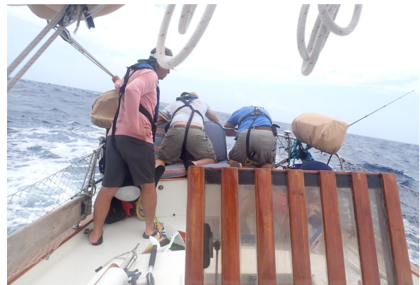
What's so interesting there, fellas? Trying to make an expedient repair to the DuoGen after it was damaged by a large vine. Fixing it would have to wait until Bocas.
