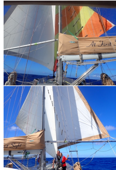
Two examples of a twizzle rig on AFS , using a spinnaker pole and the boom to pole out headsails.
