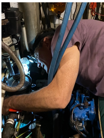
Troubleshooting the Perkins fuel system in the seaway outside Las Palmas harbor.
