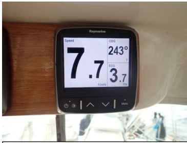
Our speed through the water was 7.7kts transiting the Strait of Gibraltar, but against a 4kt current our speed over ground (SOG) was just 3.7kts.
