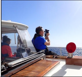
David taking a noonsite with a sextant while Vicki records the precise time of the sighting.
