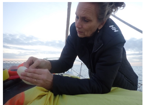
Left. Sailing on a close reach at 6kts into the sunset – until we saw a run of pinholes tracking parallel along the luff of the sail. Right. Vicki using ripstop nylon repair tape to fix the problem, at least for now. We think we may be fighting a losing battle if we see any more pinholes.
