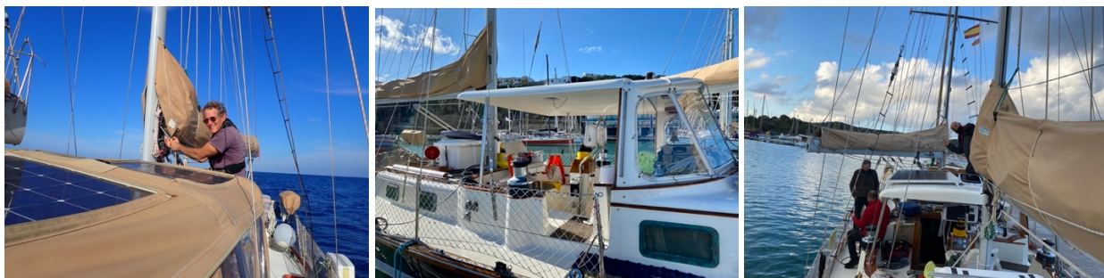
AFS, before and after her new hardtop Bimini. The 4 smaller panels produced a max of 6amps each at 24volts, and the new bigger panels produce a max of 9amps each at 38volts. The end result is the sun does a lot more charging of our batteries so we don't have to use our generator as often. And we're hoping that when summer comes, we might not have to use it at all.
