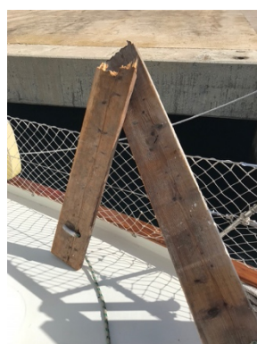
Far left: Sailor inspects our fender set up to make sure AFS stayed off the pylons. Left: This 2x12" wood fenderboard was snapped like a toothpick from the force of getting slammed against the pylons. It was sacrificial – better the fenderboard than our hull!
