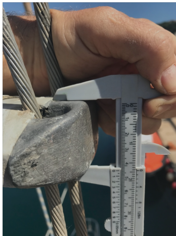
That's some nasty looking corrosion. And the fasteners were galvanically welded to the aluminum, too.
