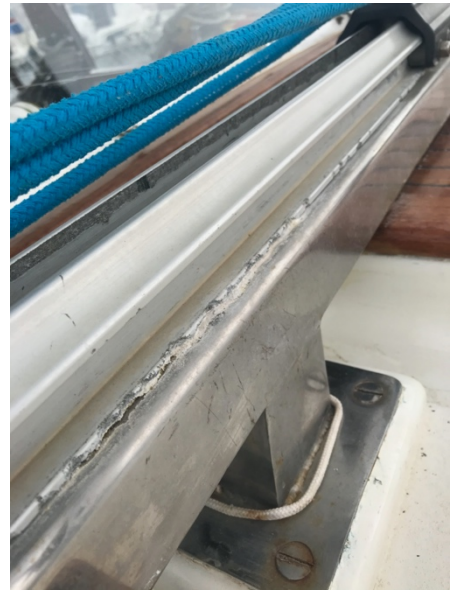
That's some nasty looking corrosion. And the fasteners were galvanically welded to the aluminum, too.
