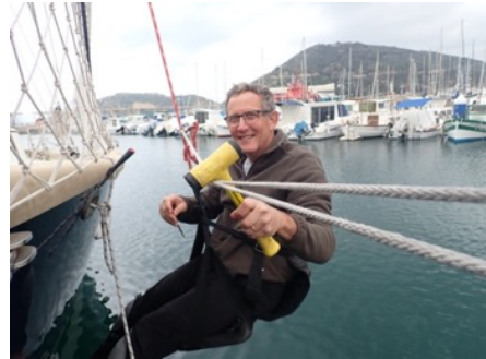
It was a team effort to remove my handiwork , the broken cleated hawse pipe, while we looked for a replacement online and waited for it to arrive. Vicki worked the inside, while I went over the side in our bos'n chair, which is normally used for going up the mast. Although we never found an identical replacement, we fortunately located a suitable substitute on eBay and worked with a nearby boatyard to install it after an agonizing 2-week delay in its arrival.
