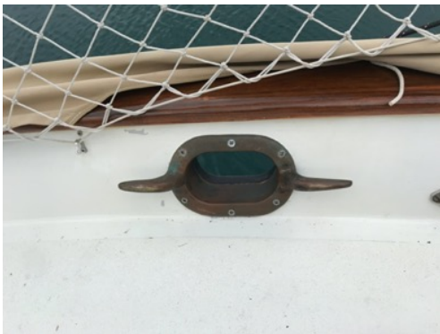
We got help from boatyard Astillero ASCAR to make reinforced fiberglass pieces to adapt our new used hawse pipes to fill in "dead space. The hardest part, really, was the emotion involved with cutting a bigger hole in the port and starboard bulwarks for the new fittings.
