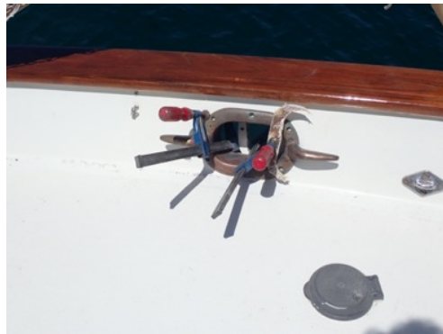
We got help from boatyard Astillero ASCAR to make reinforced fiberglass pieces to adapt our new used hawse pipes to fill in "dead space. The hardest part, really, was the emotion involved with cutting a bigger hole in the port and starboard bulwarks for the new fittings.
