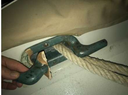
It was a team effort to remove my handiwork , the broken cleated hawse pipe, while we looked for a replacement online and waited for it to arrive. Vicki worked the inside, while I went over the side in our bos'n chair, which is normally used for going up the mast. Although we never found an identical replacement, we fortunately located a suitable substitute on eBay and worked with a nearby boatyard to install it after an agonizing 2-week delay in its arrival.
