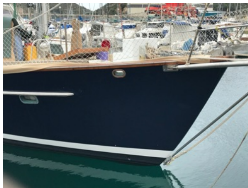
We got help from boatyard Astillero ASCAR to make reinforced fiberglass pieces to adapt our new used hawse pipes to fill in "dead space. The hardest part, really, was the emotion involved with cutting a bigger hole in the port and starboard bulwarks for the new fittings.
