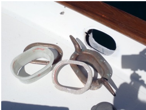
We got help from boatyard Astillero ASCAR to make reinforced fiberglass pieces to adapt our new used hawse pipes to fill in "dead space. The hardest part, really, was the emotion involved with cutting a bigger hole in the port and starboard bulwarks for the new fittings.
